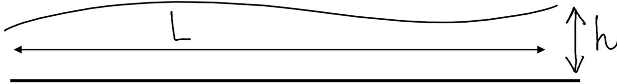
$$\rho \left( \cancel{\frac{\partial u}{\partial t}} + \underbrace{u \cancel{\frac{\partial u}{\partial x}} + v \cancel{\frac{\partial u}{\partial y}}}_{\sim U^2/L} \right) = -\frac{\partial p}{\partial x} + \mu \left( \cancel{\frac{\partial^2 u}{\partial x^2}} + \frac{\partial^2 u}{\partial y^2} \right)$$
