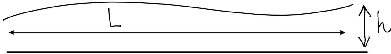
$$\frac{\partial u}{\partial x} + \frac{\partial v}{\partial y} = 0, \quad \frac{\partial p}{\partial x} = \mu \frac{\partial^2 u}{\partial y^2} \Rightarrow \phi \sim \frac{\mu U L}{h^2}$$
